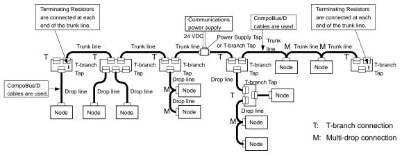
CompoBus/D cables (5-wire cables) are used for the trunk lines and drop lines.
